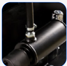
Engine heating system
